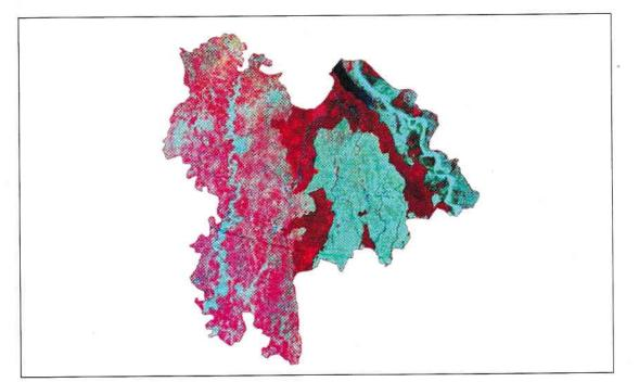
Fig. 4 Image showing the Merged Imagery of Pilibhit District extracted from the Mosaic<br/>after Data Merging of IRS P6 Data with Landsat 7 Data.<br/>IRS P6 LISS III (MSS)Landsat 7 Data.<br/>Landsat 7 ETM (PAN)[18th Nov. 2005 & 13th Oct. 2005][9th Nov. 1999 & 15th Oct. 1999]
