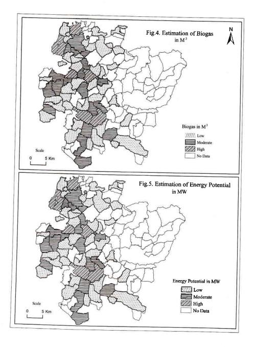
layers using ARC/GIS 9.1, using Survey of India toposheets (1:50,000 scale) and the cadastral map of Namakkal taluk. The attribute data values were added to the map layers to generate maps of village-wise biogas energy potential. The theoretical potential is presented as a thematic map of the total amount of biogas energy available in each village.
