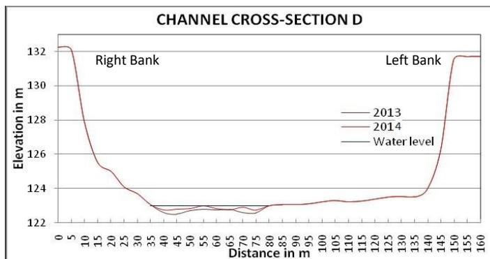
**Fig. 5. Channel Cross Section at D**
