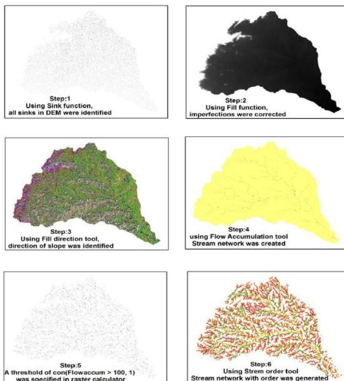
**Fig. 4. Step-by-Step Process for Extraction of Stream Network Using Hydrology Tool in ArcGIS**
