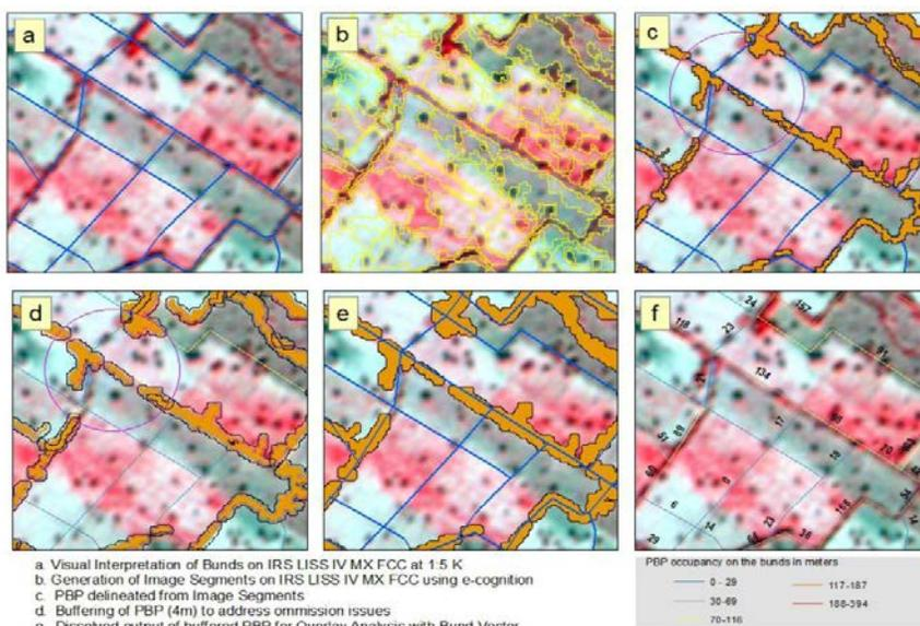
**Fig. 7. Delineation of field Peripheral Bund Plantation using OBIA on High Resolution PAN sharpened IRS imagery in Rajasthan**
