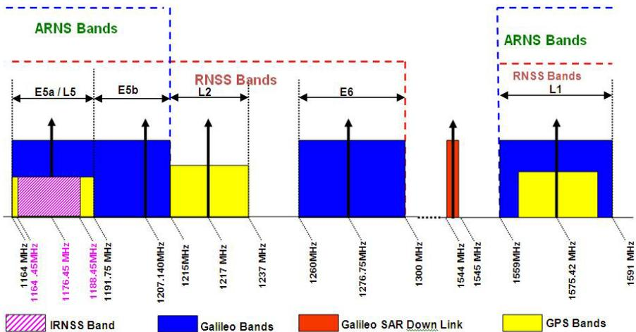
Fig. 3. IRNSS Spectrum for Radio Navigation Satellite Services in L-Band
