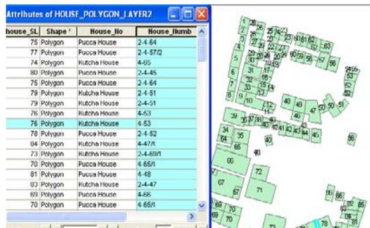
**Fig. 8. Sample of Joining of Excel Data with Polygon Feature collected through Total Station**
