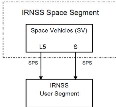
Fig. 2. IRNSS Space Segment Interface with User Segment
