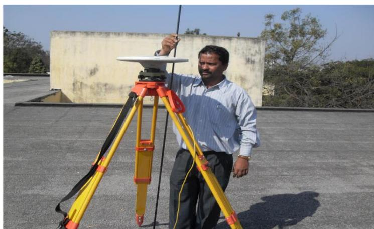
**Fig. 3. GCP observation on IISM-Top by GPS Trimble 5700**
