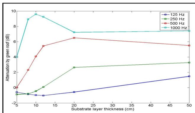
**Fig. 5: Attenuation of Noise by green roof**
